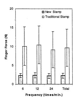
Figure 1. Variation of finger forces on each stamping frequency.
